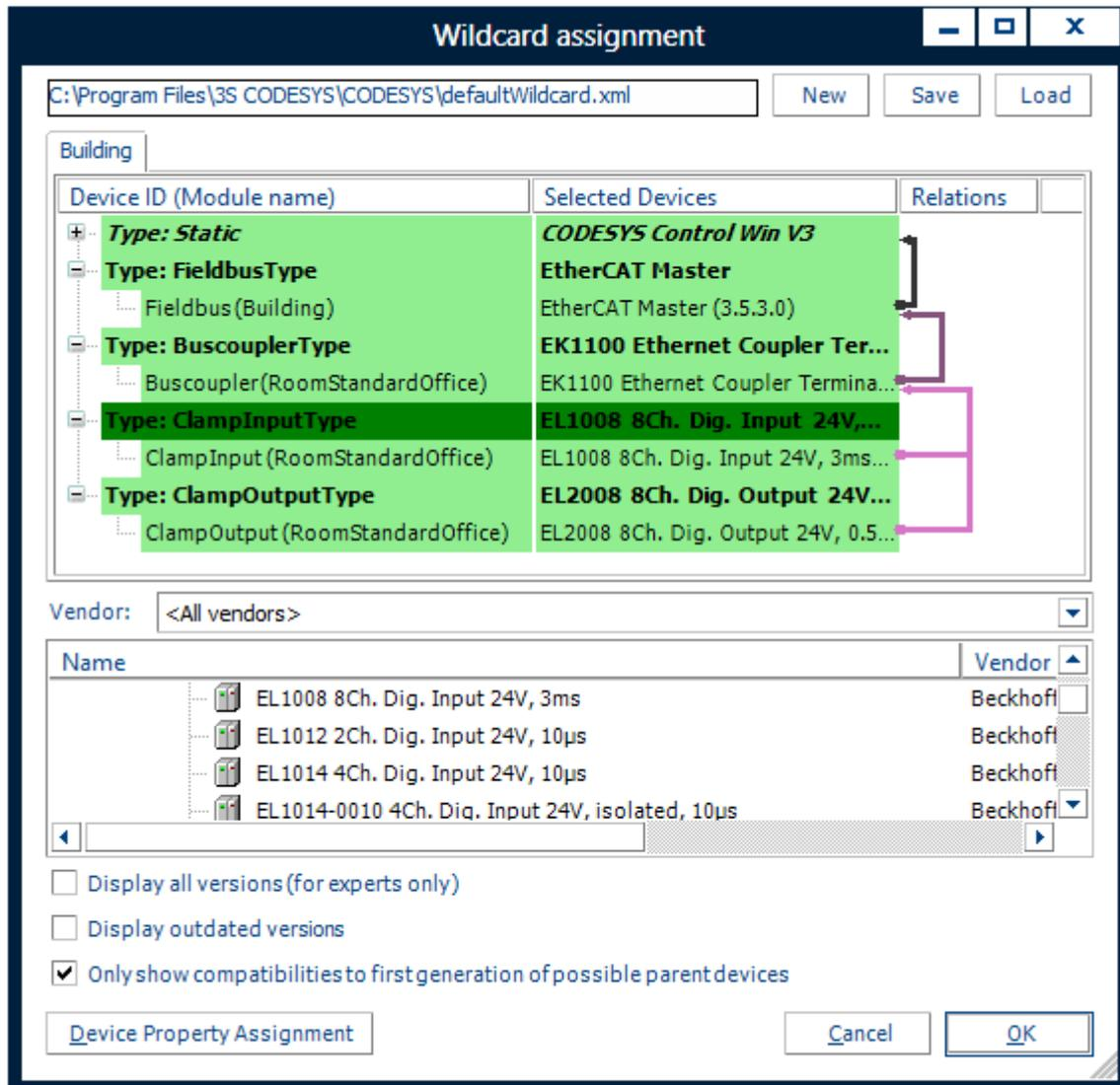
Picture 4: Assignment of module channels to devices
