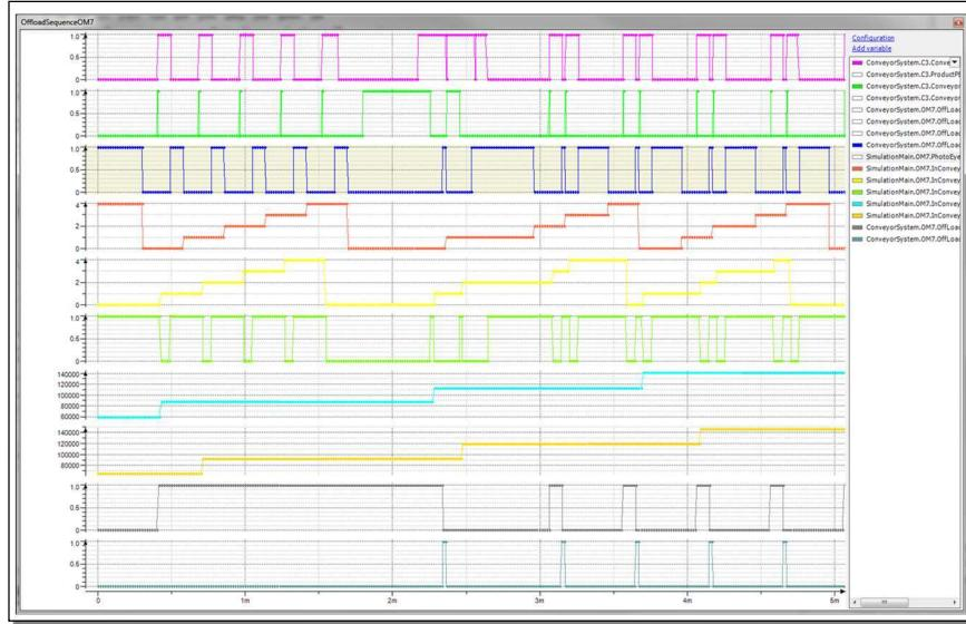
A Trace can be used to monitor the results of the simulation. And/or the simulation models themselves can monitor for the expected behavior in a fully automated test system. In this case, the traces show the handshaking between each piece of equipment, the outputs of the proximity sensors, the inputs to the motors, and the status of each conveyor simulator.
