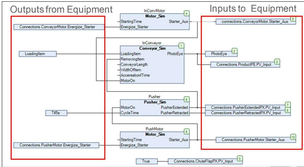
Pushing into the OffloadingModule\_SIM shows that the simulator for this module consists of two Motor simulators, a Conveyor simulator, and a Pusher simulator. Notice that the inputs to the simulators are the physical outputs of the control code. The inputs on the left are full-path names to the physical outputs in the control code, and the
