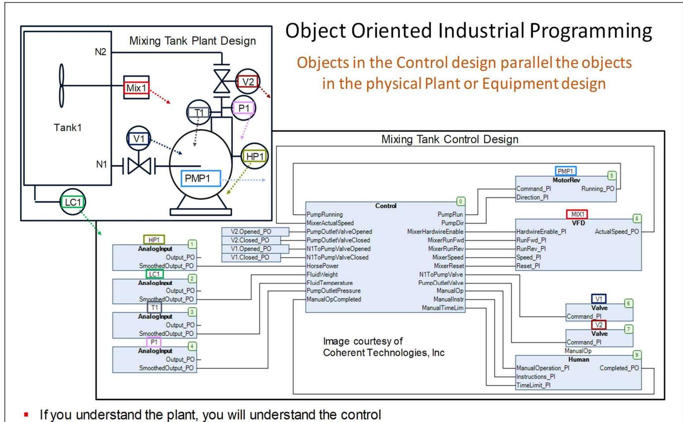
Control Objects can be designed to correspond to the objects in the plant in such a way that the control program begins to look similar to the physical plant design as shown in this graphic. Notice the one-to-one correspondence between the physical objects and the Control Objects.
