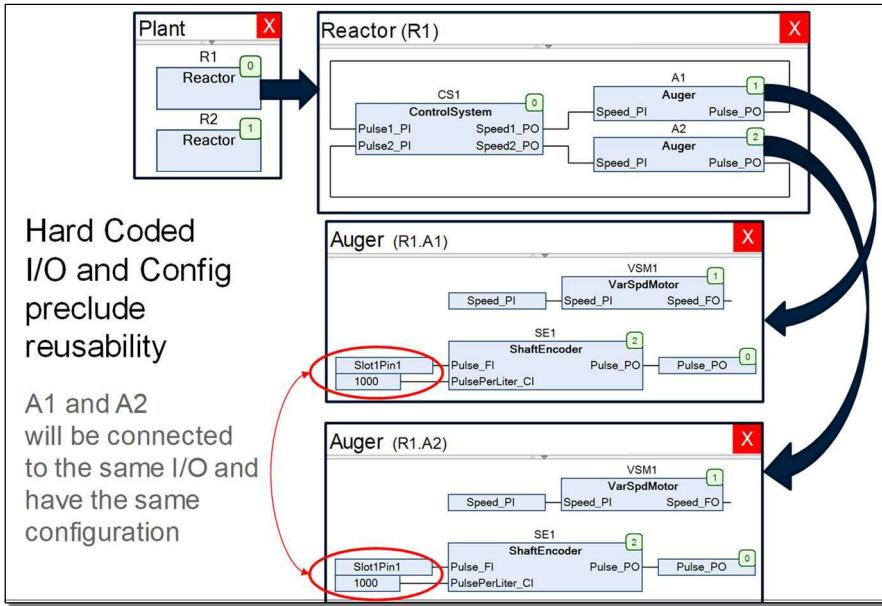
This figure shows how Abstraction, Composition, and Interfaces can be used to build a hierarchical process plant. At the top level, the Plant Program instantiates two Reactor objects, each of which have abstracted away the complexity of two Auger objects which themselves instantiate Motor and Shaft Encoder objects. The Shaft Encoder and Motor objects encapsulate all the functionality required to receive pulses from the shaft encoder and control the motor.
