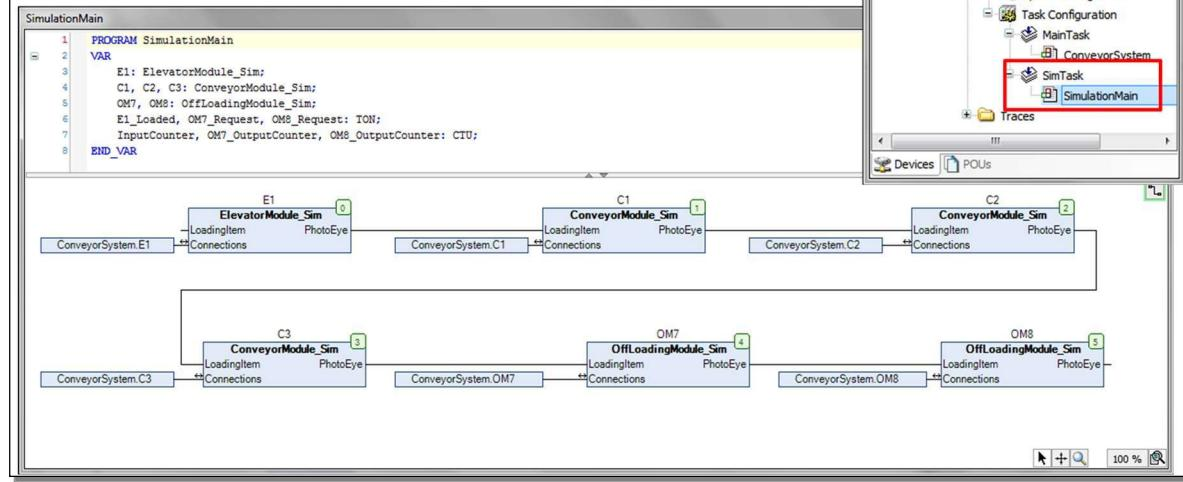
The simulation code often mirrors the control code. Here is the simulation code for the container handling system described earlier in this chapter. It contains the same blocks as the control code, except this is using the simulation
